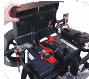
9. Open the battery box cover to the left.
