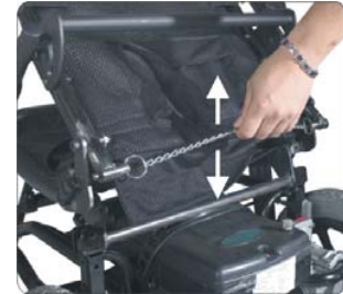
3. Pull the chain behind the seat.
